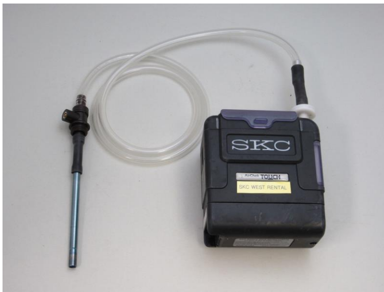
Figure 2. Air Sampling Assembly of SKC AirChek Touch Pump, Constant Pressure Controller, and Single Tube Holder
