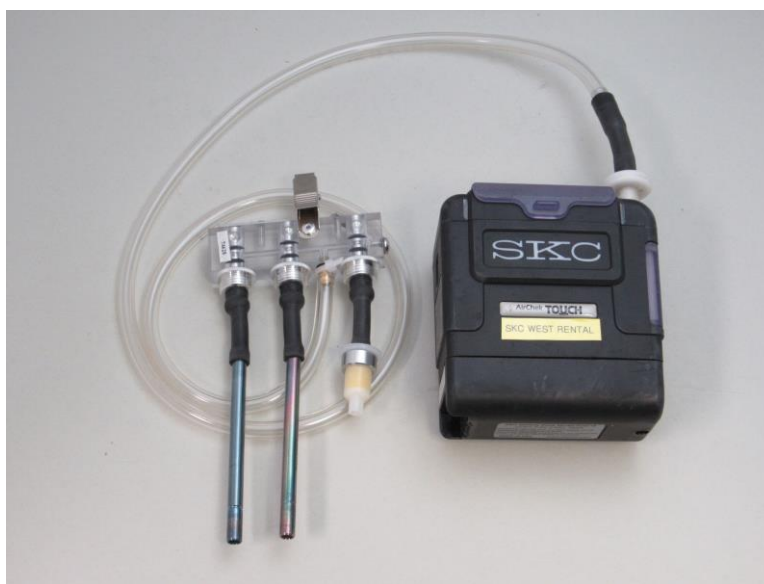
Figure 1. Air Sampling Assembly Using SKC AirChek Touch Pump, and Tri-tube manifold
