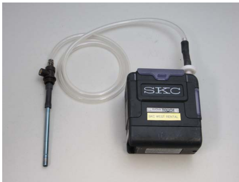
Figure 2. Air Sampling Assembly of SKC AirChek Touch Pump, CPC, and Single Tube Holder
